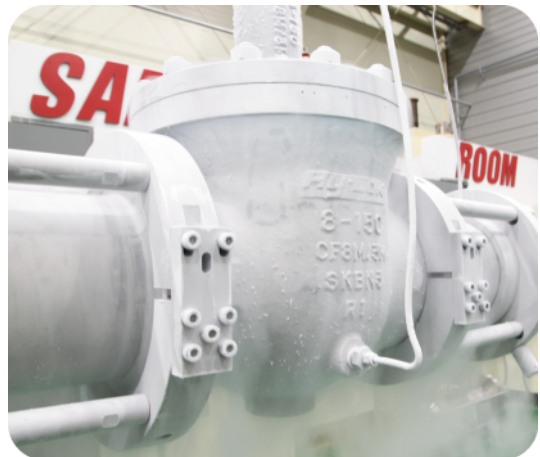
Cryogenic testing on an 8 in. Top Entry Ball Valve
