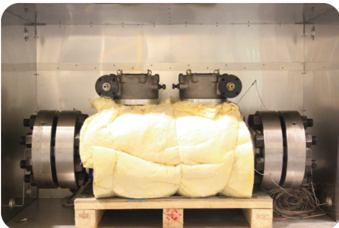
High temperature testing on an 6 in. Double Block & Bleed Valve
