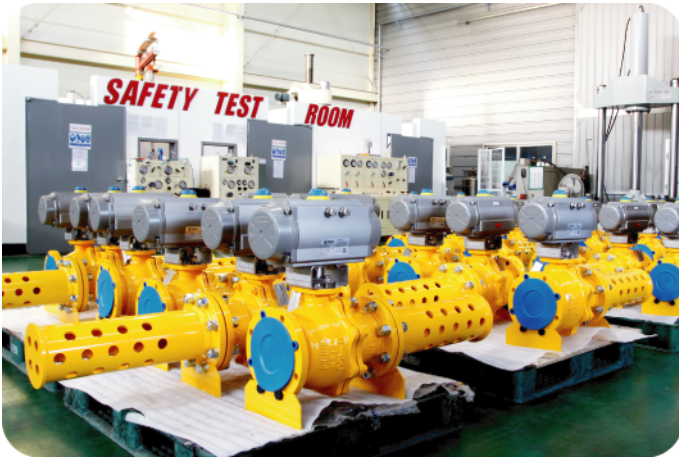
Testing Facilities for valves up to 12 in.
